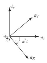
$$\begin{aligned} & \text{soit}: & e(t) = NSK\omega'M_o\left(u\,\cos(\omega't) + v\,\sin(\omega't)\right) \\ & \text{ou}: & e(t) = V_0\cos(\omega't) + V_{\frac{\pi}{2}}\cos(\omega't) & \text{tels que}: \begin{cases} & V_0 = NKSM_o\omega'u \\ & V_{\frac{\pi}{2}} = NKSM_o\omega'v \end{cases} \end{aligned}$$
